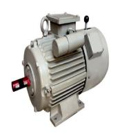
Brake Motor is combination of three phase or single phase Squirrel Cage Induction Motor with Electro-Magnetic Disc Brake (A.C.) when power is switched off with ordinary motor, the rotating part will stopped after some time but if brake motor is used rotating mass will stop instantaneously. All Brakes are mounted at non-driving end of motor, braking disc is mounted directly on motor shaft. Brakes are directly acting, no lever or links are required.
